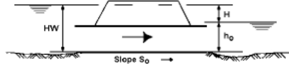
SUBMERGED OUTLET CULVERT FLOWING FULL
