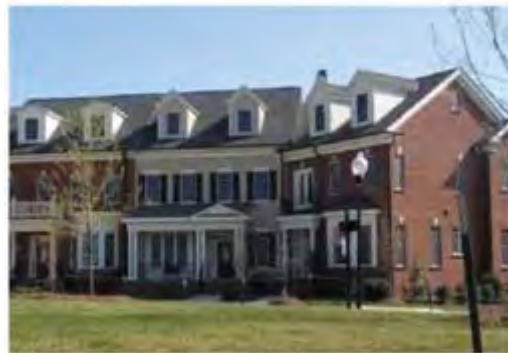
YES: The primary building material is continued around the corners. Note the middle unit changes material to avoid monotony
